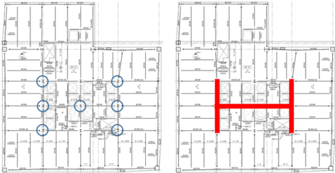
Figure 12 | Existing Core Columns and Replacement Shear Wall (Courtesy of Heller Manus)
